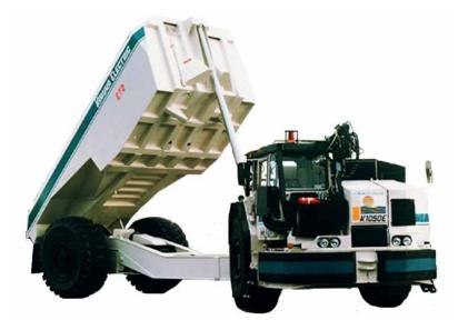
Kiruna Electric ED is the only electric truck in range of 35 and 50 ton capacity for underground haulage. In the normal haulage the truck is powered by an overhead trolley line (no exhaust fumes), when leaving the trolley line a small TIER III diesel engine (~80 kW) is activated. The diesel engine is mainly used when you have no access to the trolley line e.g. loading and dumping stations.
