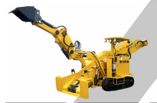
**The crawler borne Häggloaders are electro-hydraulic driven,** trackless digging-arm or back-hoe loaders, particularly suitable for use in drifts and tunnel with cross section from 8 m<sup>2</sup> and upwards.
