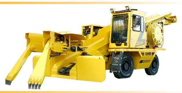
The wheel borne Häggloaders are rubber tyred electro-hydraulic driven, trackless loaders with a unique dual digging arm system. Available in two models 7HR and 10HR.
