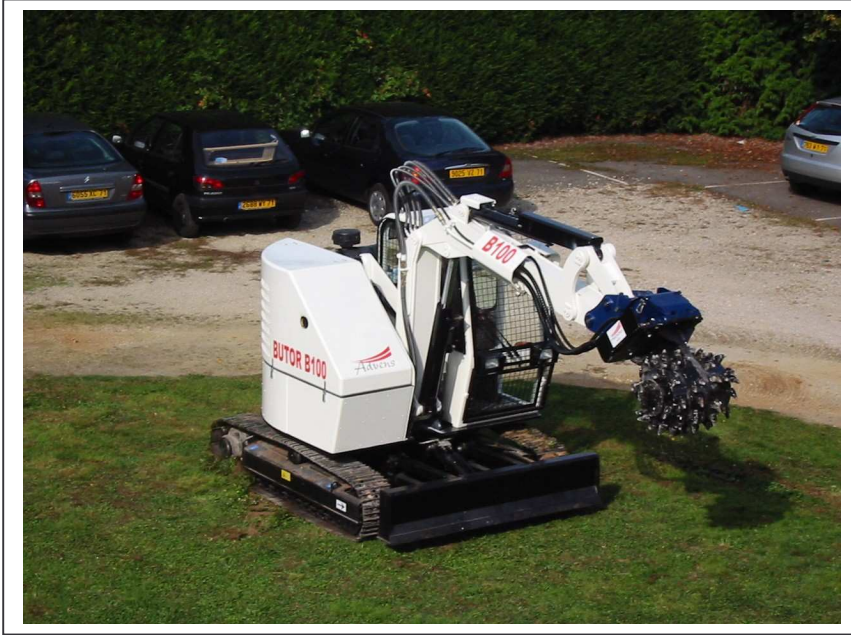
B 100 T with demolition head
