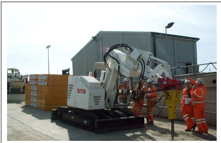
TEM with Hydraulic Rock Breaker on rotary arm
