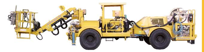
ANFO Charging equipment. High speed and high charging density for face and up holes.
