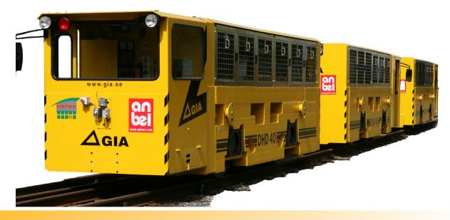
The diesel hydrodynamic (DHD) locomotives are available in the range of 15 to 45 tonnes.
