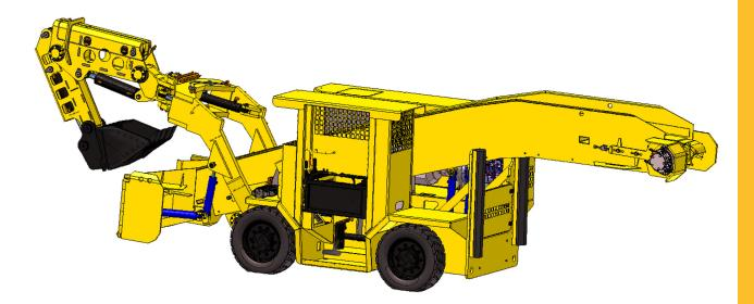
The wheel borne Häggloaders are rubber tyred electro-hydraulic driven, trackless loaders with a back-hoe digging system. Available in two models 7HR-B and 10HR-B.
