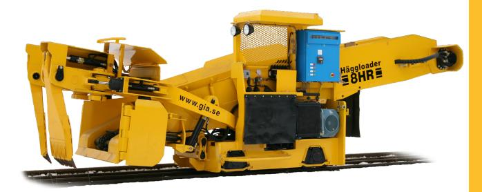
The railborne Häggloaders are electro-hydraulic driven loaders with a unique dual digging arm system designed to operate efficiently in narrow or limited work areas.
