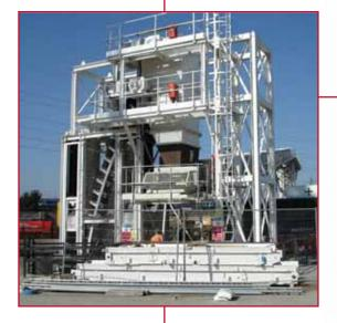
HAC technology has solved many high capacity, steep angle conveying problems, up to and including vertical lifts. The Joy system employs standard idlers and rollers and a simple, but unique, sandwich principle, that overcomes the limitations typically encountered with many traditional methods of conveying.
