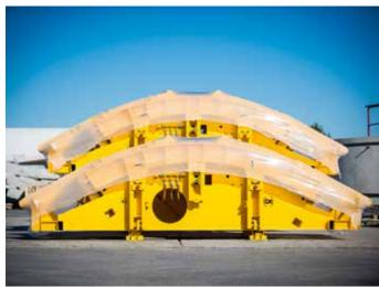
CBE Group has successfully taken part in the development of **segment moulds for tunnels of all dimensions:** 1 to 17 m diameter, 18 to 60 cm thickness, 3 to 17 tons.
