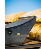
CBE Group's expertise is based on its ability to design a long-lasting mould which will produce a high quality segment. Each mould is designed to produce at least 1,500 segments.
