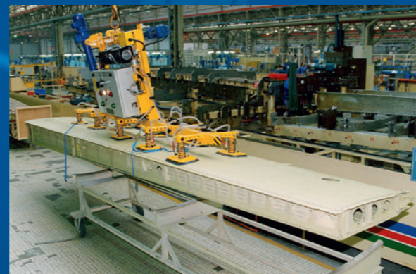
Vacuum beam for aluminium plate application
