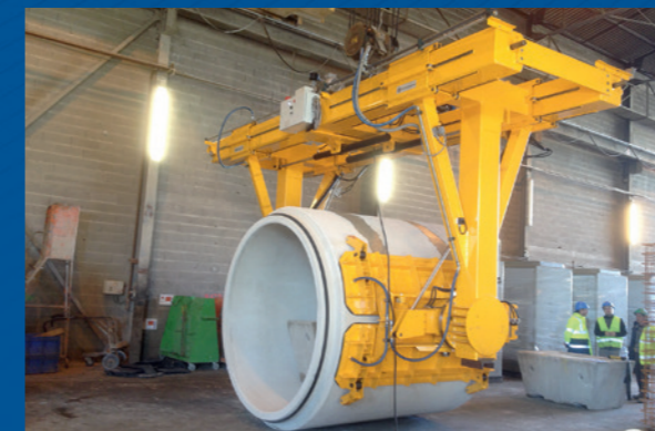
Demoulding turning beam
